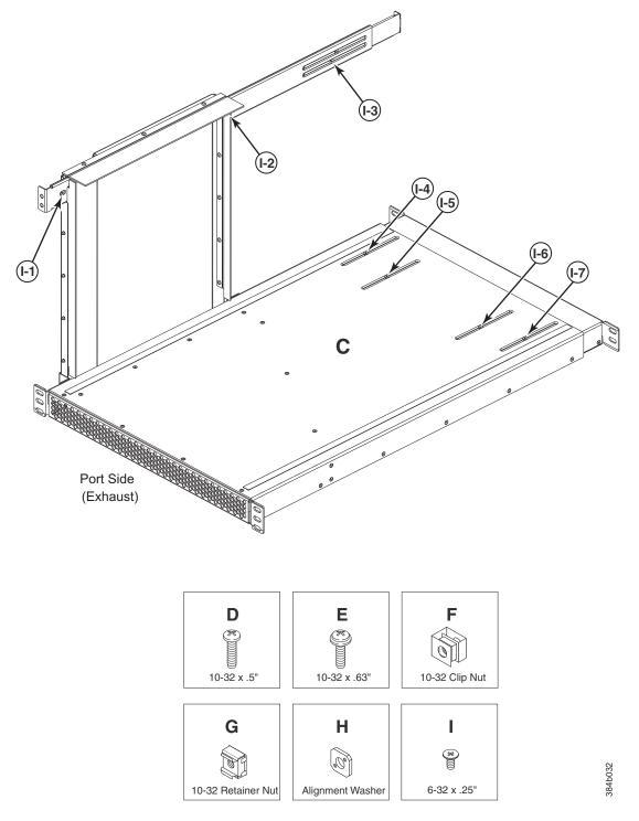
Figure 6. Port-side exhaust kit assembly for 27 to 31 in. (68.58 to 78.74 cm) cabinets
